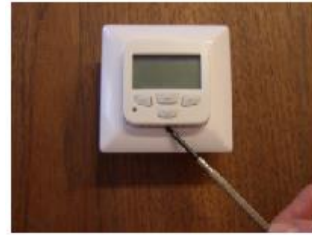
Figure 7: Operator bezel removal
