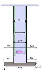
Fasten the height adjustment rails (4 pcs) with M5X20 screws (8 pcs) as shown.
