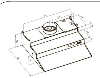
Attach the hood ( A= 500 or 600 mm ) to the furniture with installation accessories. The installation height between the cooker hood and hob level should be at least 500 mm.
