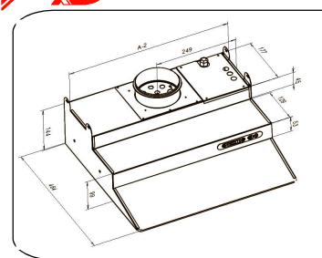
Attach the hood ( A= 500 or 600 mm ) to the furniture with installation accessories. The installation height between the cooker hood and hob level should be at least 500 mm.
